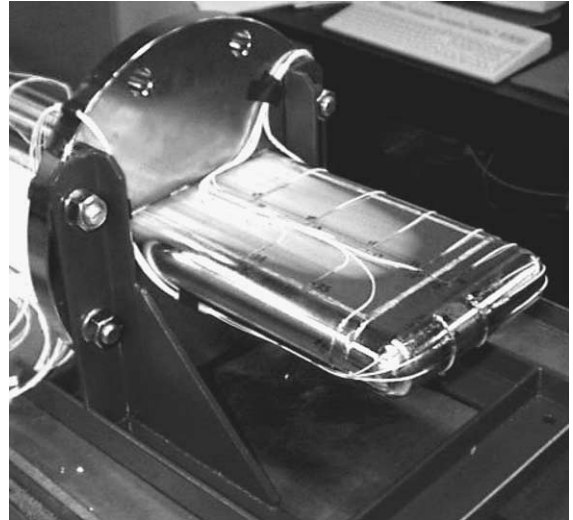
Fig. 12. Prototypic-shape target with strain sensors.
